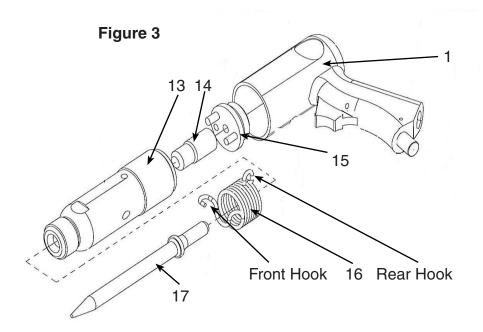
**NOTE:** The threads inside the Cylinder (13) are plastic. Do not exert too much twisting pressure or they can be damaged. The Cylinder should easily twist into the Housing (1) until snug. See **Figures 2 & 3**
